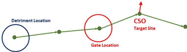
This document provides an overview of modelling a simple single gate installation, considering the target CSO, the gate location and a supplementary upstream detriment location. It will explain how to add the network components, define starting values for the system and set up the CENTAUR™ RTC protocols to replicate system behaviour.
