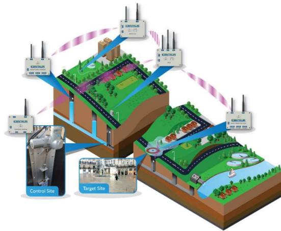
Our proprietary AI system manages flow control devices using a **SENSE-THINK-ACT** approach to optimise operation at the target overflow, enabling the reduction of spill frequency and duration.
